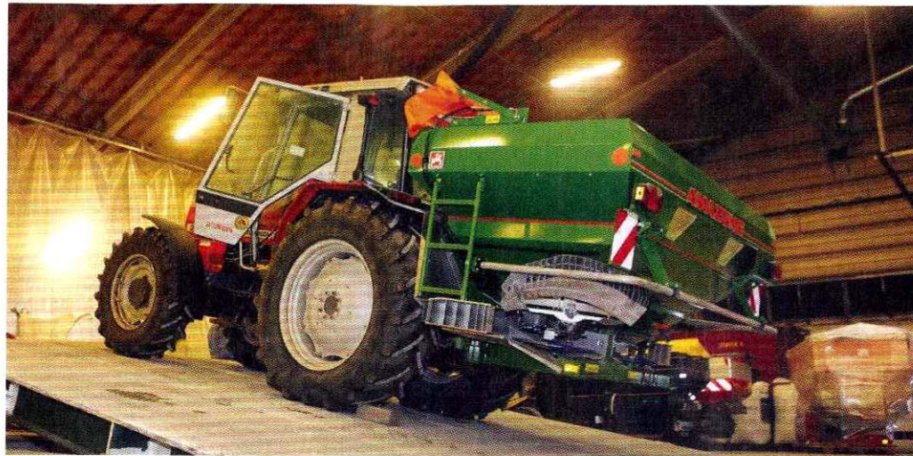
Above: Amazone's ZA-M Ultra is the only one to alter the width by changing the position of the vanes.
