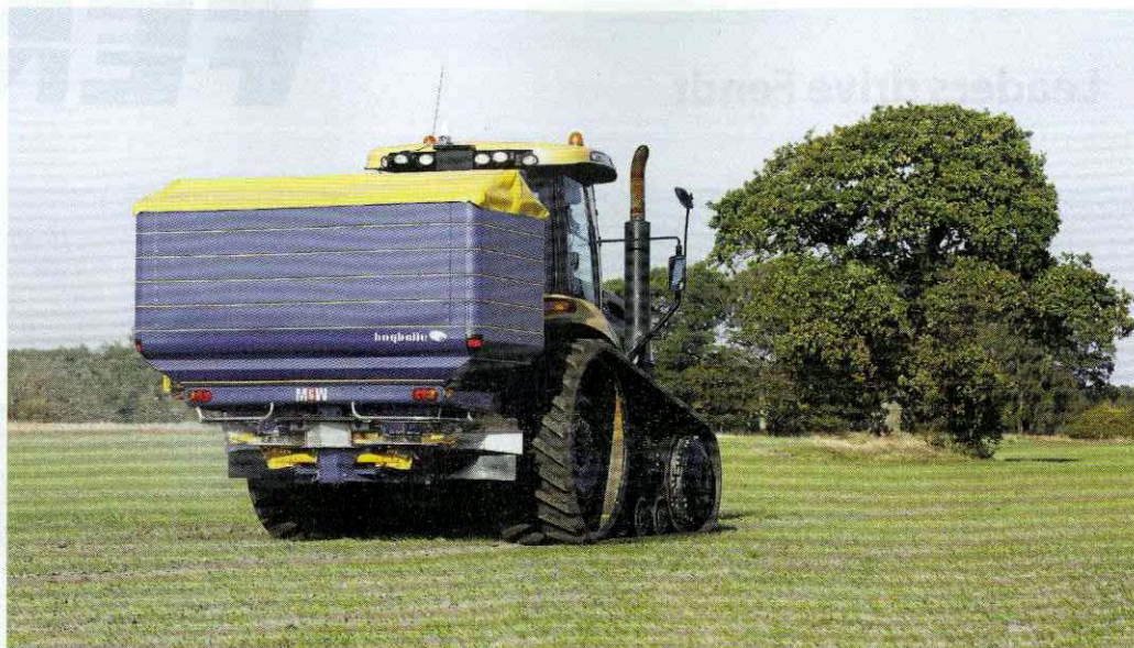
Bogballe claims the 5,500-litre M6W is the biggest linkage-mounted fertiliser spreader on the market.
