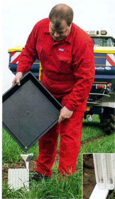
An accessory kit lets you pattern-test the spreader in the field. It's easy to use.
