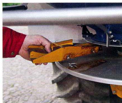
Disc vanes lock into one of several positions.
