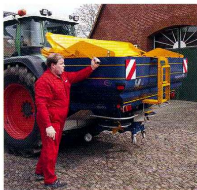
The hopper cover folds manually, with hydraulic operation optional. Also an extra, the rear folding ladder is useful. Storage wheels let the empty spreader be moved around on smooth floors.
