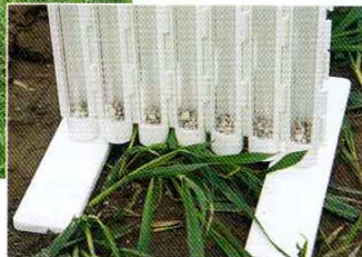
An accessory kit lets you pattern-test the spreader in the field. It's easy to use.
