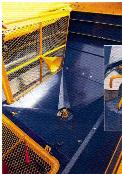
Standard grids can be doubled if lumps are a problem. Two agitators (inset) are covered by a cone when the grids are down, which force side entry and so minimise granule damage.
