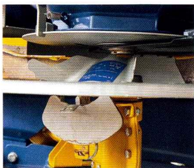
A single disc pictured from the side. During calibration a section is removed, the disc is positioned under an outlet and locked, and a chute is swung into place. Hopper emptying used the same procedure.
