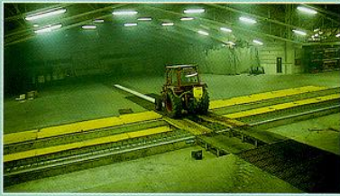
The machine passes over two rows of funnelled containers in the test hall. Weighing is carried out automatically.
