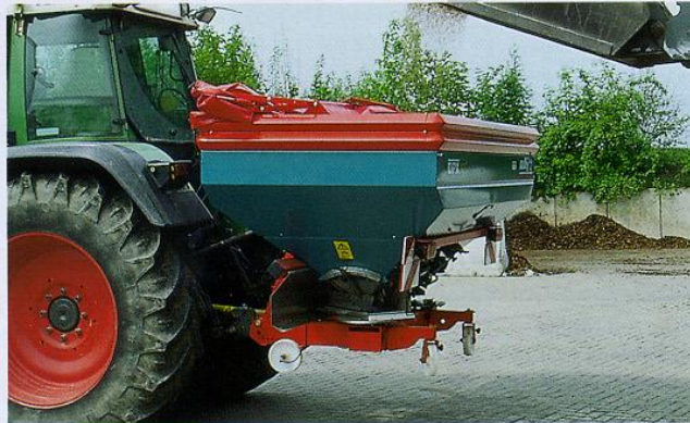
Sulky DPX expert: After adjusting the fertiliser/disc drop point, the DPX came in at under 10% CoV.
