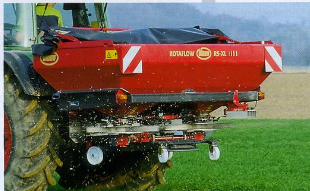
Vicon RS-XL: Like the Sulky, the Vicon spreader needed adjusting to achieve its sub-15% CoVs.
