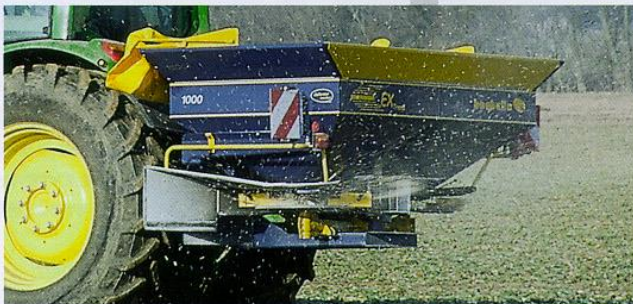
Bogballe/KRM EX trend: The test results speak for themselves. The EX trend's CoV figure never topped the 10% benchmark.
