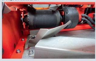
**Belt application** is a distinguishing Bredal feature. It is hydraulically driven and automatically adjusts to the driving speed.
