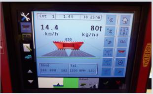
**This shows** belt and disc speeds, etc. A small cut-out view from GPS or a camera is seen at the very bottom. The spreader can also be controlled on a different ISOBUS screen.
