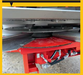
Spreading discs are usually belt-driven, but the latest feature on the list of optional accessories is this hydraulic drive. It can be used for headland spreading on both sides and can be disengaged during operation without having to stop the discs. This avoids having to maintain the PTO shaft and check the belt tightener. It does require the tractor to have a hydraulic pump that can supply at least 120 litres a minute, however. The drive also uses two hydraulic outlets.
